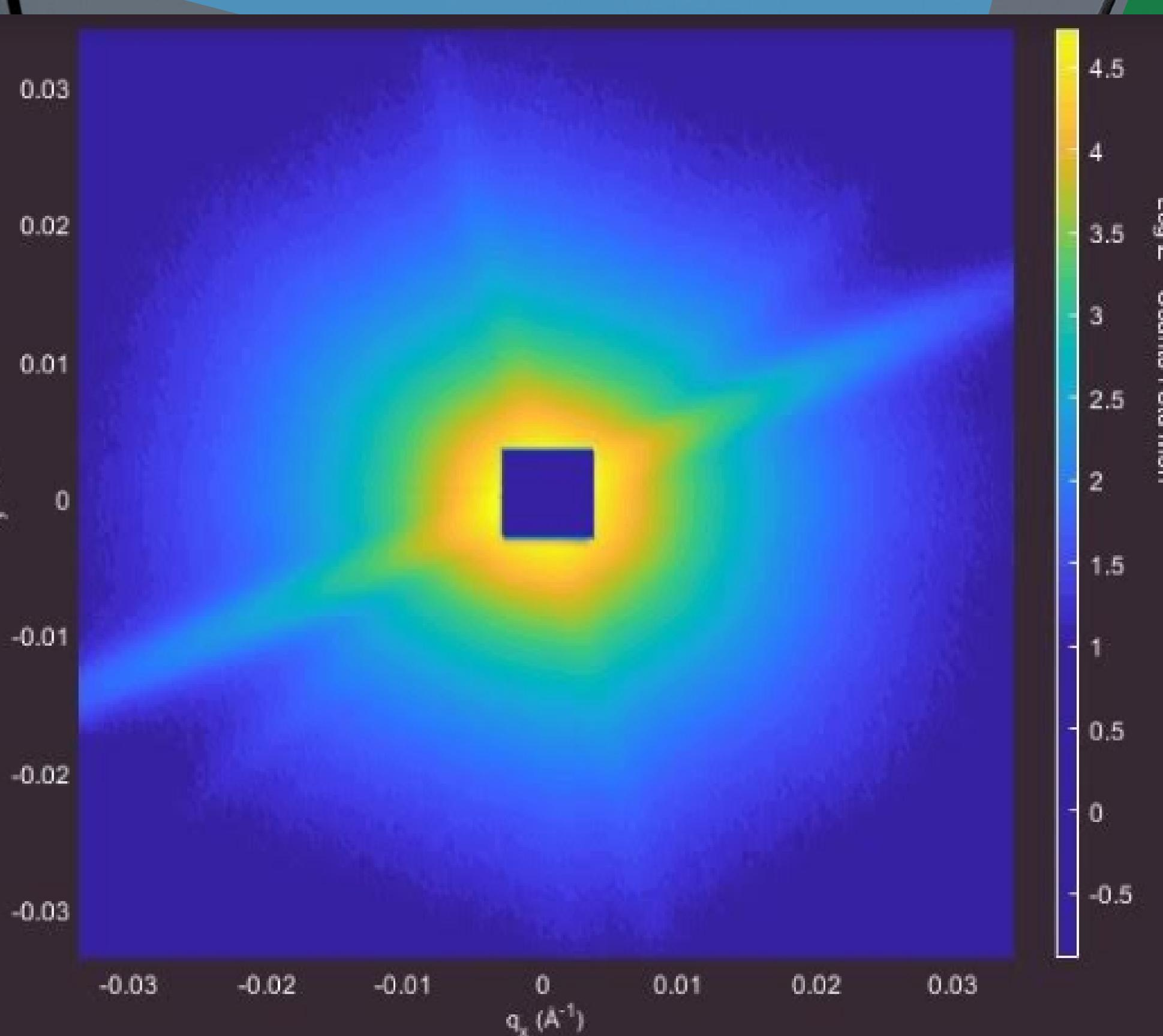
The image showcases the Small Angle Neutron Scattering intensity (2D plot) measured at  $T = 150$  K for a  $\text{Tb}_{4.925}\text{La}_{0.075}\text{Si}_2\text{Ge}_2$  sample. This temperature value corresponds to the Griffith's phase, which takes place between  $T_C = 105$  K and below the  $T_G = 190$  K.
