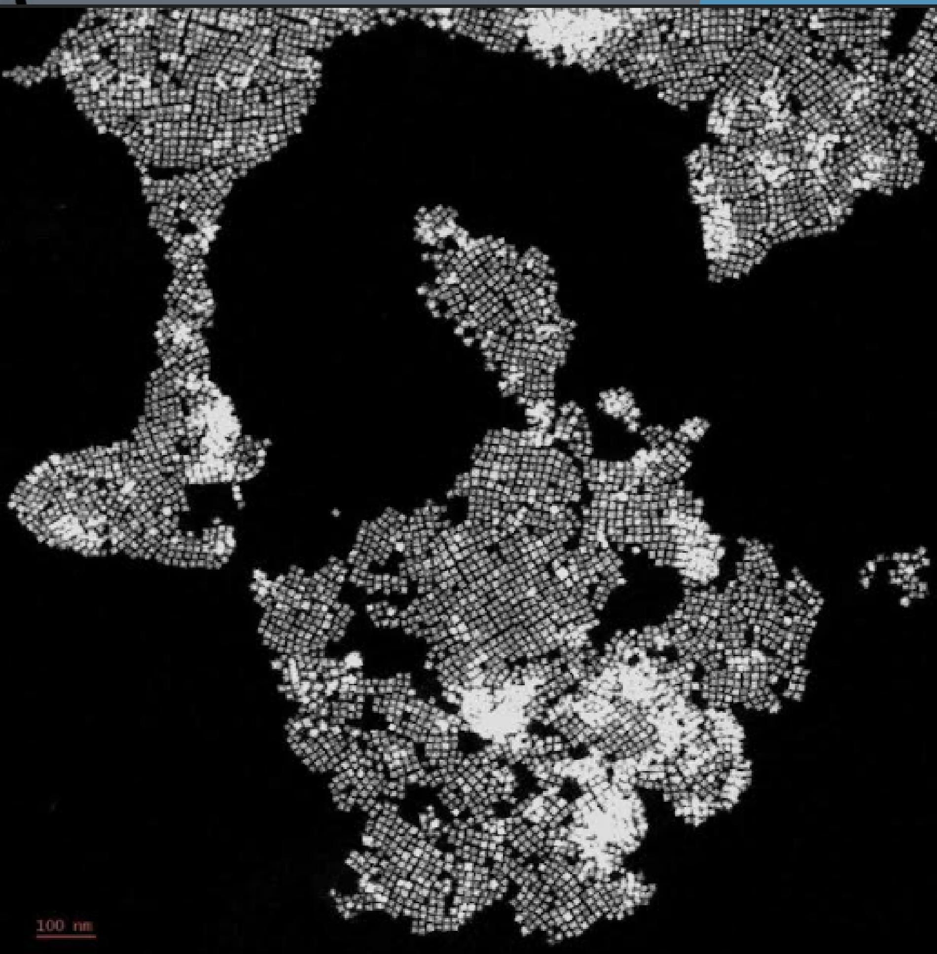
The image shows an arrangement of magnetic core/shell  $\text{Fe}_3\text{O}_4@\text{CoFe}_2\text{O}_4$  nanoparticles.
