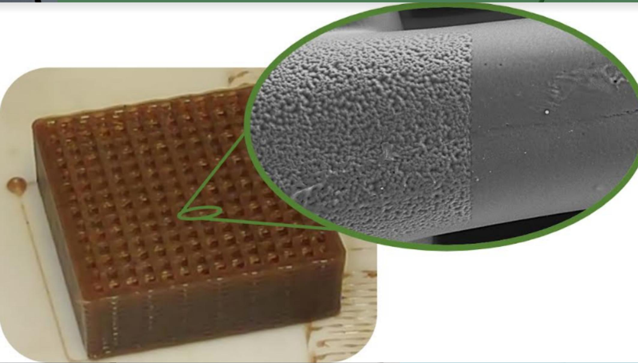
Selective texturing on the rods surface of a woodpile-like 3D structure made of iron oxide nanoparticles dispersed in a biopolymer matrix after been high-field exposure. The structure has been 3D printed using a direck ink writting additive manufacturing technique (robocasting).
