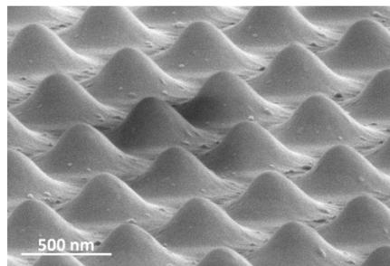
Figure 1. SEM image of the Terfenol-D pillars deposited over a Si substrate.
