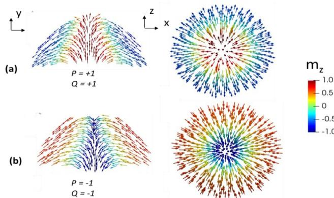
Figure 1. (a-b) Chiral quasi-skyrmion magnetization configurations in permalloy caps. P and Q stand for the polarity and the chirality of the skyrmion respectively.
