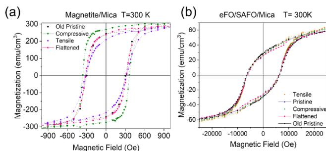
Figure 1: Magnetization response for different bending states of the magnetite (a) and epsilon iron oxide (b) thin films at room temperature.
