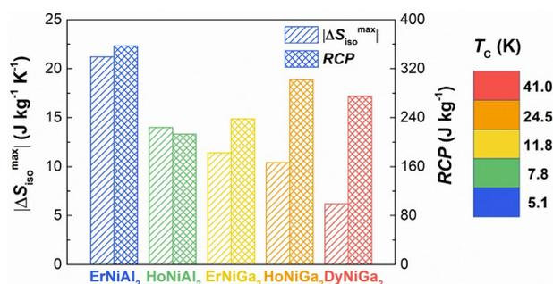
Fig.1  $|\Delta S_{iso}^{max}|$  and the relative cooling power (RCP) under  $\Delta H$  of 0-5 T for the studied compounds
