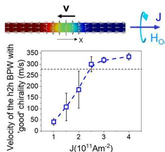
**Figure 1.** The average velocity of a head-to-head BPW driven by a spin-polarized current in a Ni nanowire far from the ends of the nanowire as a function of the current density.
