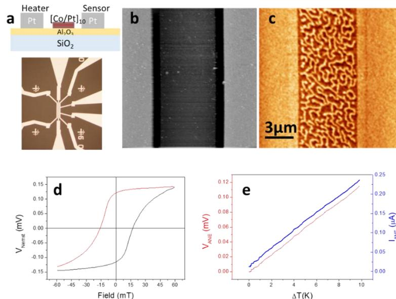
Figure 1: a) Scheme and optical microscope image of the device. b) AFM topography and c) magnetic signal measured by MFM of the device. d) Hysteresis loop of the Nernst voltage as a function of the magnetic field. e) Voltage and current obtained from the device as a function of the thermal gradient.
