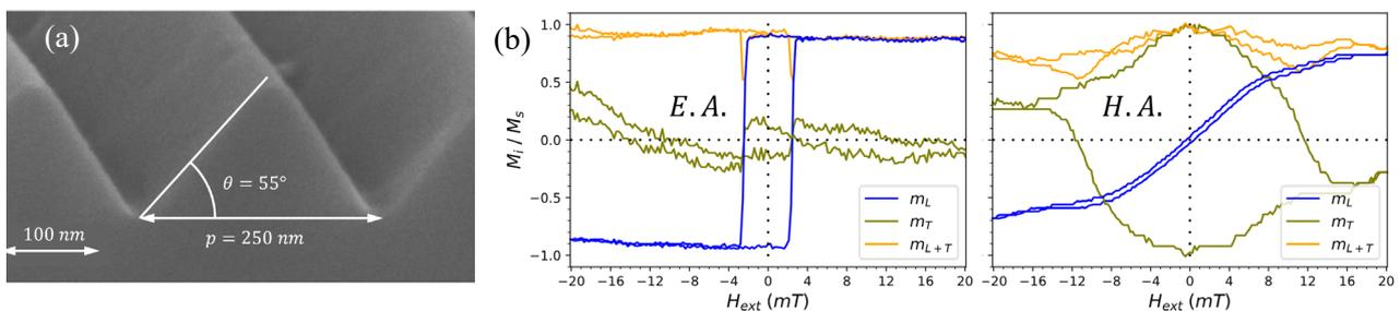
Figure 1. (a) SEM image of nanopatterned V-groove silicon substrate before Py film deposition. (b) Anisotropic behavior of a 15nm width V-groove Py, showing longitudinal (blue) and transversal (green) magnetization in measured hysteresis loops at the easy (left) and hard (right) in-plane magnetization axes of the sample.
