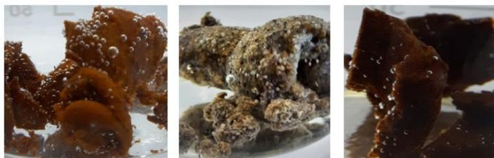
Figure 1. Polyurethane composites with different magnetic nanoparticles in their composition.
