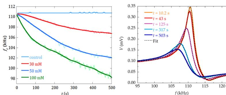
**Figure 1:** a) Temporal evolution of the resonance frequency of the magnetoelastic sensor as the reaction progresses (for different concentration of reactants in the reaction). b) Temporal evolution of the resonance curves during the reaction for 30 mM reactants and corresponding numerical fits.
