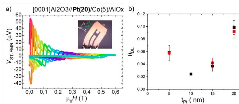
Fig. 1. a). Field sweep ST-FMR spectra. The RF frequency varies from 1 to 22 GHz. The inset shows a ST-FMR device. b)  $\theta_{DL}$  from  $Al_2O_3//Pt/Co/AlO_x$  samples as a function of Pt thickness for both crystallographic directions,  $\Gamma K$  and  $\Gamma M$ .
