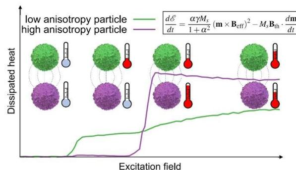
**Figure 1.** Heat generated in a system consisting of two interacting nanoparticles with different anisotropies. Both particles show switching behavior as soon as the excitation field amplitude overcomes their anisotropy barrier. The heat generation tends to become more uniform with increasing excitation fields.
