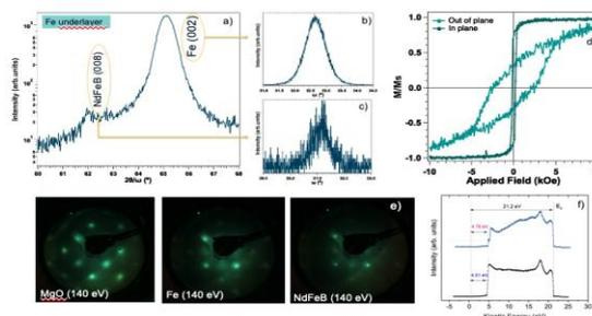
Figure 1: a) XRD pattern of a NdFeB thin film with an Fe underlayer, b) rocking curve measurement of Fe (002), c) rocking curve of NdFeB (008), d) room temperature hysteresis loop, e) LEED pattern of MgO substrate, Fe buffer layer and NdFeB film, f) work function measurements of Fe buffer (bottom) and NdFeB film (top).
