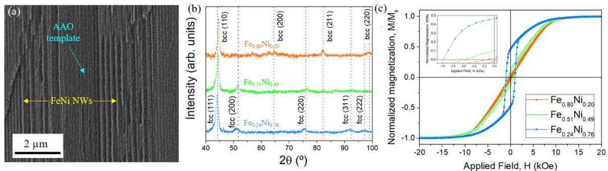
Fig. 1. (a) SEM image showing an array of FeNi NWs in AAO template; (b) and (c) XRD patterns and room temperature hysteresis loops for arrays of NWs with composition Fe<sub>0.80</sub>Ni<sub>0.20</sub>, Fe<sub>0.51</sub>Ni<sub>0.49</sub> and Fe<sub>0.24</sub>Ni<sub>0.76</sub>.
