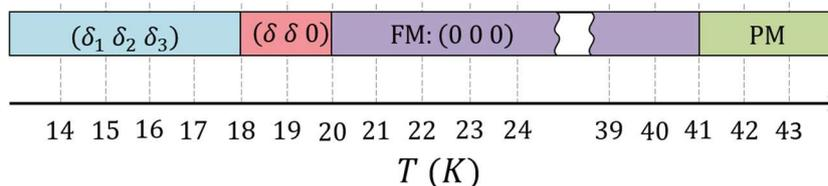
Fig. 1. Phases present in  $\text{MnCr}_2\text{O}_4$  together with their phase transition temperatures. Green: paramagnetic order, purple: ferrimagnetic order, pink: conical order with  $\vec{k}_{S1} = (0.62(1), 0.62(1), 0)$ , blue: conical order with  $\vec{k}_{S2} = (0.660(3), 0.600(1), 0.200(1))$ .
