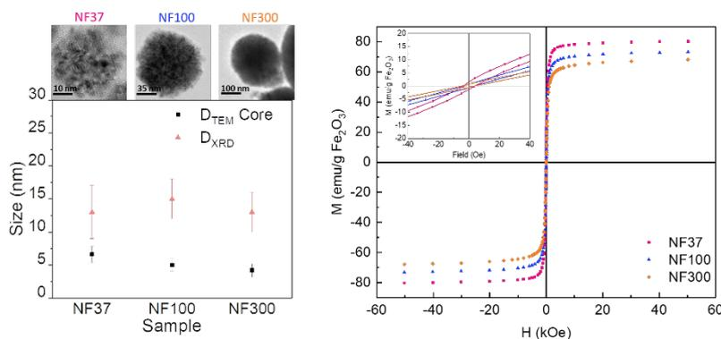
Figure 1. Left panel shows the core diameters obtained from TEM (black squares) and XRD (red triangles) data for the three samples, together with the corresponding TEM images of the NF aggregates at the top of the panel. Right panel shows hysteresis loops at 300K. The inset corresponds to the enlarged region between -40 and +40 Oe.
