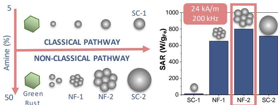
**Figure 1.** SAR values of single core (SC) and nanoflowers-like (NF) nanocrystals obtained by classical and non-classical pathways. The amount of amine controls the formation mechanism.
