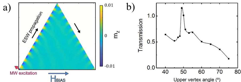
**Figure.** a) Snapshot of an edge spin wave propagated through both sides on a 2 micron side YIG triangle with a local microwave sinusoidal excitation perpendicular to the left side. b) Transmission coefficient of the ESW propagation through the upper vertex topology, showing a distinct increment for upper vertex angles in the 49°-50° range.
