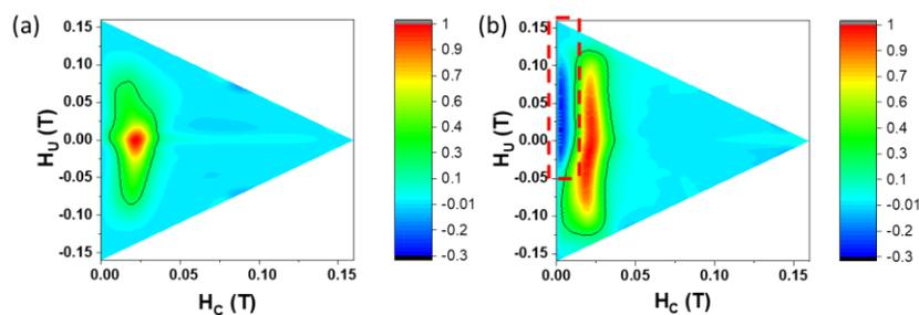
Figure 1. FORC diagrams. (a) Array of Fe<sub>20</sub>Ni<sub>80</sub> nanowires and (b) array of chemically modulated Fe-Ni nanowires.
