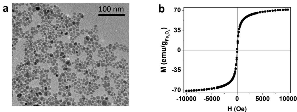
Figure 1. (a) Transmission electron microscopy (TEM) micrograph of Fe<sub>3</sub>O<sub>4</sub> MNPs dispersed in water.
