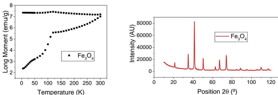
Figure 1. a) ZFC-FC curves of an iron oxide sample. b) Corresponding XRD pattern.
