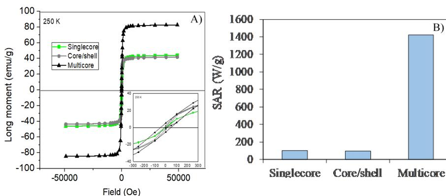
**Figure 1.** A) Magnetization hysteresis loops at RT in emu/gNP B) optimum SAR values for dyes degradation.
