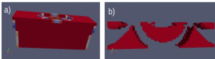
Figure 1: Illustrative result of an optimization where a) is obtained as local minimum with the algorithm in [2] and b) as global minimum (reduction of the same cost function by another 10%) with the hybrid algorithm.
