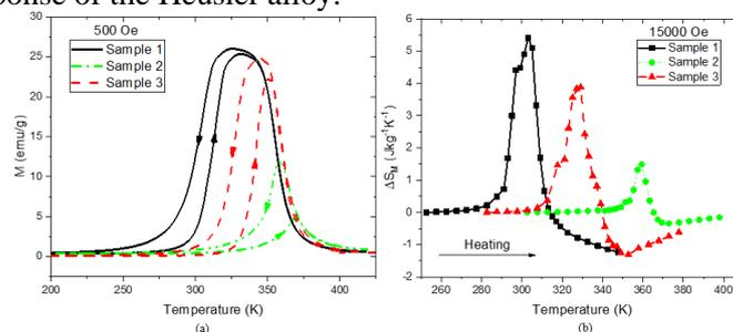
Figure 1(a): Temperature dependence of magnetization and (b) Isothermal entropy change ( $\Delta S_{iso}$ )
