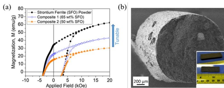
Fig. 1. (a) First and second quadrants of the hysteresis loops of recycled strontium ferrite (SFO) powder and composites with different contents of SFO particles embedded in polymer matrix (magnetization scales with the PM particles content making possible tuning the PM properties). (b) SEM image showing the circular cross section of the filament (65 wt% of SFO). Inset shows pictures of the printed object.
