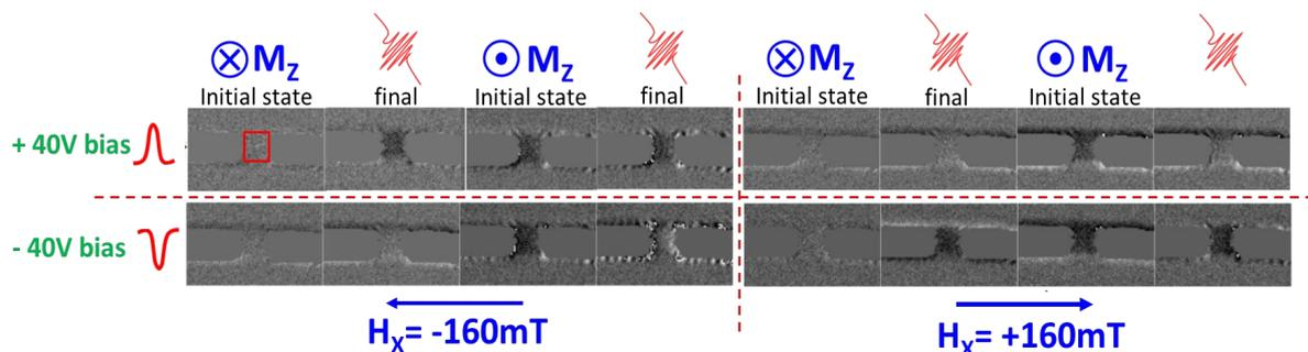
Figure 1. Polar MOKE images of Co (1nm) sample for different combination of polarities of the ps electric pulse and the external In-plane magnetic field to verify the presence of spin orbit torque driven magnetization reversal.
