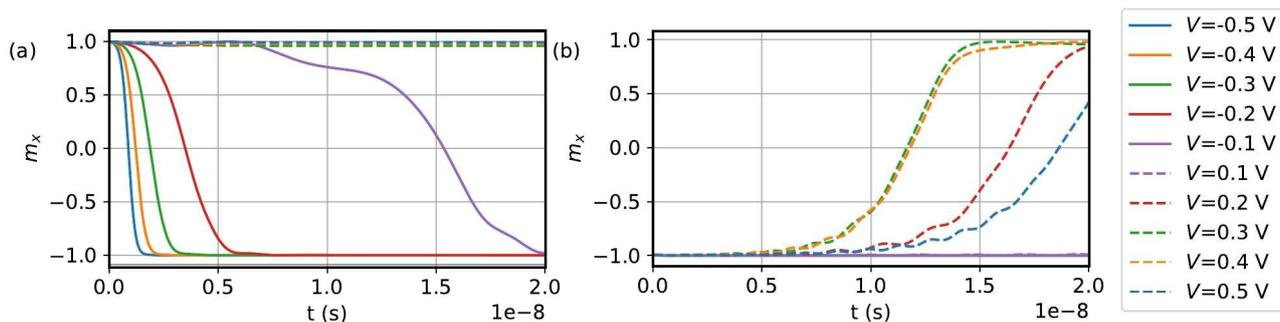
Fig. 1: Magnetization dynamics in an asymmetric magnetic tunnel junction. Subfigure (a) shows the parallel to antiparallel magnetization reversal for negative voltages, (b) shows the antiparallel to parallel switching direction for positive voltages.
