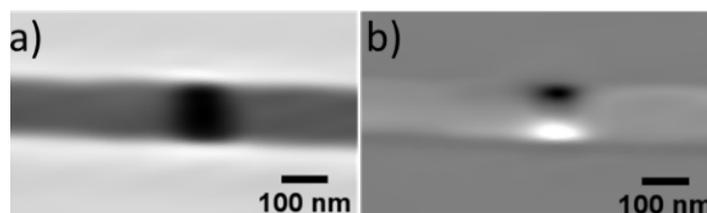
Figure 1 a) Reconstructed amplitude ptychographic XAS image at the Fe L3 edge of a Permalloy cylindrical nanowire of 140 nm of diameter with a chemical modulation ( $\text{Fe}_{80}\text{Ni}_{20}$ ) of 100 nm in length (dark region). b) Reconstructed XMCD ptychographic image of a). The curling magnetization is evidenced by the dark and white bipolar contrasts.
