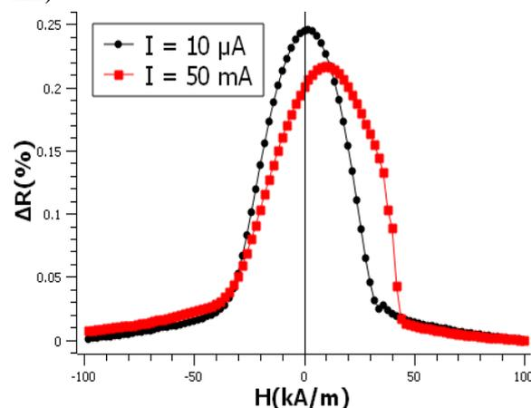
**Figure 1.** AMR curve without (black) and with (red) current effects being taken into account. A symmetry break has been generated in the positive field region of the red curve, which results in a steeper slope (higher sensor sensitivity).
