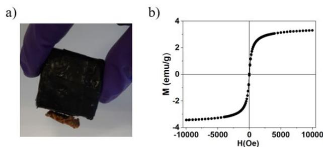
Figure 2. a) Magnetic composite attracted by a magnet. b) Superparamagnetic behaviour of the composite.
