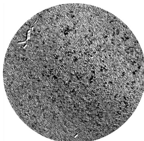
MTXM imaging of Co nanowires ( d=35 nm, L=150 nm)
