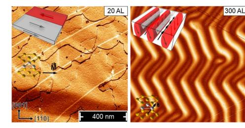
Spin-polarized STM images of the magnetic domain structure of Gd films on W(110) at film thickness of 20 atomic layers (left) and 300 atomic layers (right). Schematic representations are shown in the upper left.
